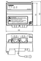
Please consider when attempting to install the WJ200 series that by attaching any of the WJ-ECT, WJ-PB or WJ-PN option, the inverter D (depth) size will increase by 26.3 mm regardless of the inverter capacity.
